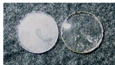
Fig. 34 Photographic images of unloaded zeolite L monolayers on a glass substrate. Left: uncoated monolayer. Right: similar sample coated with Columbia Resin 39 (CR39).
